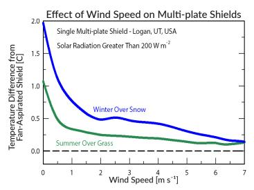
Naturally-aspirated shields are subject to significant measurement errors when wind speeds are less than  $3 \, \text{m s}^{-1}$ . Errors increase when snow covers ground surface.
