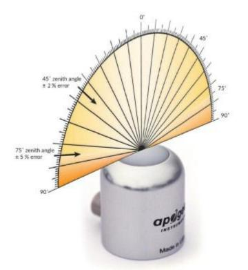
Directional, or cosine, response is defined as the measurement error at a specific angle of radiation incidence. Directional error for Apogee SU-200 series UV-A sensors is approximately ± 2 % and ± 5 % at solar zenith angles of 45° and 75°, respectively.
