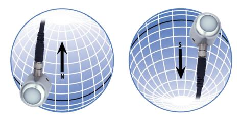
In addition to orienting the cable to point toward the nearest pole, the sensor should also be mounted such that obstructions (e.g., weather station tripod/tower or other instrumentation) do not shade the sensor. **Once mounted, the black cap should be removed from the sensor.** The black cap can be used as a protective covering for the sensor when it is not in use.
