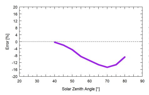
Mean cosine response of four Apogee UV-A sensors. Cosine response was calculated as the relative difference of UV-A sensors from the mean of replicate reference UV-A sensors deployed outdoors. These data are the average of the AM and PM response.
