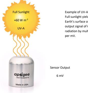
Example of UV-A measurement with an Apogee UV-A sensor. Full sunlight yields UV-A radiation on a horizontal plane at the Earth's surface of approximately 60 W m<sup>-2</sup>. This yields an output signal of 6 mV. The signal is converted to UV-A radiation by multiplying by the calibration factor of 10 W m<sup>-2</sup> per mV.
