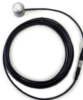
Inline cable connectors are installed 25 cm from the head
