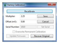
After clicking the 'Recalibate' button the user will be prompted to cover the sensor. Place a dark cap over the sensor and wait for the real-time PFD reading to settle at zero. Click OK.
