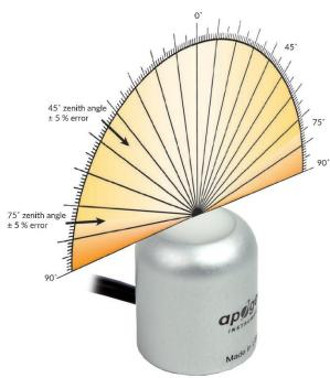
Directional, or cosine, response is defined as the measurement error at a specific angle of radiation incidence. Error for Apogee SQ-600 series Extended Range PFD Sensor is approximately ± 2 % and ± 5 % at solar zenith angles of 45° and 75°, respectively.
