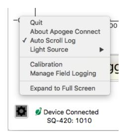
Note the **'Light Source'** function is not necessary for the SQ-626. The SQ-626 is calibrated for use under LED light sources; therefore, this function is not necessary for the SQ-626. The function is designed to give increased accuracy for the SQ-420.
