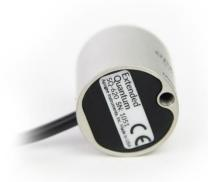
A sensor's model number and serial number are located on the bottom of the sensor. If the manufacturing date of a specific sensor is required, please contact Apogee Instruments with the serial number of the sensor.
