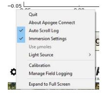
Clicking **'Calibration'** will display the factory calibrated multiplier and offset values. These values are saved in firmware and can be recovered by clicking the 'Recover Original' button. Deriving a new calibration multiplier and offset is accomplished by clicking the 'Recalibrate' button. This is applicable if users want to calibrate the sensor to their own specific light source. Note that a reference PFD value of the light source is required to complete a recalibration.
