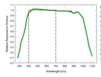
Mean spectral response measurements of x six replicate Apogee SQ-600 series Extended Range PFD Sensors. Spectral response measurements were made at 10 nm e increments across a wavelength range of 300 to 1100 nm in a monochromator with an attached electric light source. Measured spectral data from each PFD sensor were normalized by the measured spectral response of the monochromator/electric light combination, which was measured with a spectroradiometer
