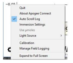
Note **'Light Source'** is not a selectable option. The SQ-626 is calibrated for use under LED light sources; therefore, this function is not necessary for the SQ-626. The function is designed to give increased accuracy for the SQ-420.
