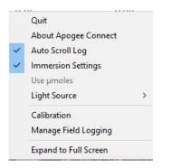
Clicking **'Calibration'** will display the factory calibrated multiplier and offset values. These values are saved in firmware and can be recovered by clicking the 'Recover Original' button. Deriving a new calibration multiplier and offset is accomplished by clicking the 'Recalibrate' button. This is applicable if users want to calibrate the sensor to their own specific light source. Note that a reference PFD value of the light source is required to complete a recalibration.
