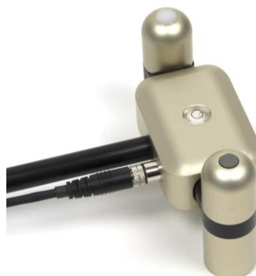
Cable connectors are attached directly to the head.
