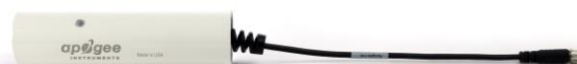
When sending sensors in for calibration, only send the short end of the cable and half the connector.
