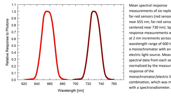
Mean spectral response measurements of six replicate red far-red sensors (red sensor is centered near 655 nm, far-red sensor is centered near 730 nm). Spectral response measurements were made at 2 nm increments across a wavelength range of 600 to 800 nm in a monochromator with an attached electric light source. Measured spectral data from each sensor were normalized by the measured spectral response of the monochromator/electric light combination, which was measured
