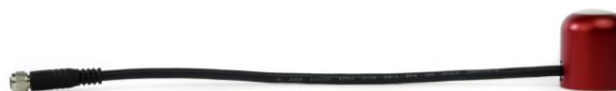
When sending sensors back for recalibration, only send the section of cable that is hard-wired to the sensor. The section of cable with the pigtail is not required.
