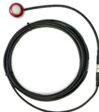
Inline cable connectors are installed 30 cm from the sensor head (pyranometer pictured).
