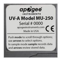
A sensor's model number and serial number are located on a label on the backside of the handheld meter.
