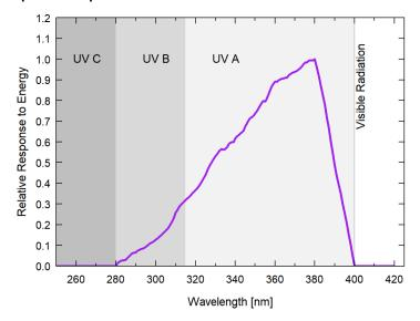
Spectral response estimate of Apogee MU series UV-A meters. Spectral response was modeled from sensitivity of the photodetector and transmittance of the diffuser.
