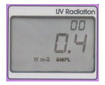
The LCD display consists of the total number of logged measurements in the upper right hand corner, the real-time UV measurement in the center, and the selected menu options along the bottom.
