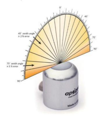
Directional, or cosine, response is defined as the measurement error at a specific angle of radiation incidence. Directional error for Apogee SU-200 series UV-A sensors is approximately  $\pm$  2 % and  $\pm$  5 % at solar zenith angles of 45° and 75°, respectively.
