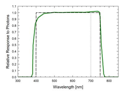
Mean spectral response measurements of four replicate Apogee MQ-600 series ePAR Sensors. Incremental spectral response measurements were made at 10 nm increments across a wavelength range of 370 to 800 nm in a monochromator with an attached electric light source.
