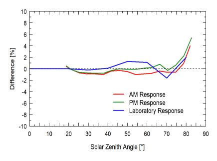
Mean directional (cosine) response of seven Apogee series quantum sensors. Directional response measurements were made on the rooftop of the Apogee building in Logan, Utah. Directional response was calculated as the relative difference of quantum sensors from the mean of replicate reference quantum sensors (LI-COR models LI-190 and LI-190R, Kipp & Zonen model PQS 1). Data were also collected in the laboratory using a reference lamp and positioning the sensor at varying angles.
