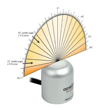
Directional, or cosine, response is defined as the measurement error at a specific angle of radiation incidence. Error for Apogee MQ-600 series Extended Range PFD Sensor is approximately  $\pm$  2 % and  $\pm$  5 % at solar zenith angles of 45° and 75°, respectively.
