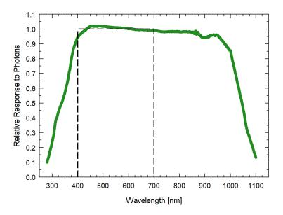
Mean spectral response measurements of six replicate Apogee MQ-600 series Extended Range PFD Sensors. Spectral response measurements were made at 10 nm increments across a wavelength range of 300 to 1100 nm in a monochromator with an attached electric light source. Measured spectral data from each PFD sensor were normalized by the measured spectral response of the monochromator/electric light combination, which was measured with a spectroradiometer.
