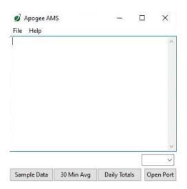
To establish communication, make sure the meter is plugged into your computer using the AC-100 communication cable. To connect click the dropdown menu button and "COM#" options will appear. For more details on how to figure out which COM is the right one, watch our video.
