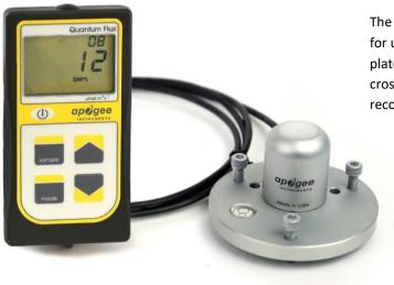
The AL-100 leveling plate is recommended for use with the MQ-620 (AL-100 leveling plate pictured). To facilitate mounting to a cross arm, the AL-120 mounting bracket is recommended.
