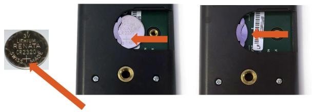
The positive side (designated by a "+" sign) should be facing out from the meter circuit board.
