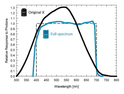
Mean spectral response measurements of six replicate Apogee SQ-100X (original X) and MQ-500 (full-spectrum) series quantum sensors. Spectral response measurements were made at 10 nm increments across a wavelength range of 300 to 800 nm with a monochromator and an attached electric light source. Measured spectral data from each quantum sensor were normalized by the measured spectral response of the monochromator/electric light combination, which was measured with a spectroradiometer.
