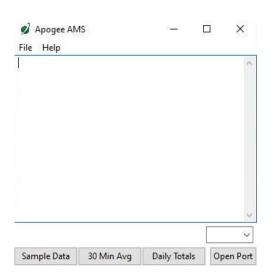
To establish communication, make sure the meter is plugged into your computer using the AC-100 communication cable. To connect click the dropdown menu button and "COM#" options will appear. For more details on how to figure out which COM is the right one, watch our video.
