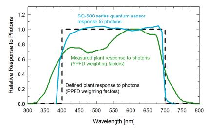
Defined plant response to photons (black line, weighting factors used to calculate PPFD), measured plant response to photons (green line, weighting factors used to calculate YPFD), and SQ-500 series quantum sensor response to photons (sensor spectral response).
