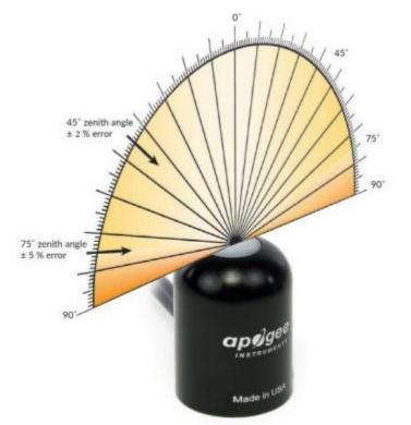
Directional (cosine) response is defined as the measurement error at a specific angle of radiation incidence. Error for Apogee SQ-100 series quantum sensors is approximately  $\pm 2$ % and  $\pm 5$  % at solar zenith angles of 45° and 75°, respectively.
