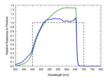
Spectral response of updated line quantum sensor spectral response graph (in green) vs. the original line quantum sensor response (in blue). For information on effects on accuracy, see the spectral error table on page 15 of this manual.
