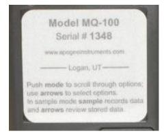
A sensor's model number and serial number are located on a label on the backside of the handheld meter.
