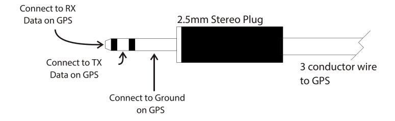
The MC-100 accepts standard RS-232 level communications (NEMA 0183 output V 2.0 or greater). Not all GPS devices output standard RS-232 levels. Check with the manufacturer of the GPS device to determine if you require a level translator (adaptor) cable to work with RS-232. GPS port BAUD rate should be set to 4800.
