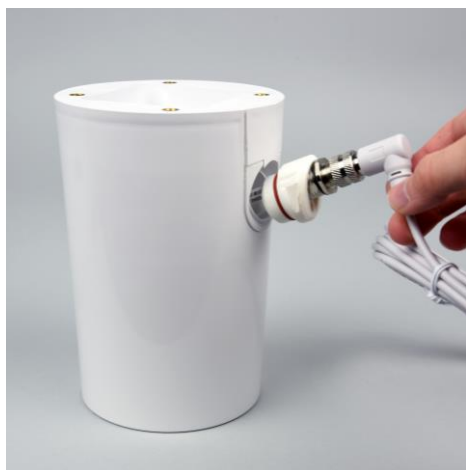
Push the EE08 into adapter port.
