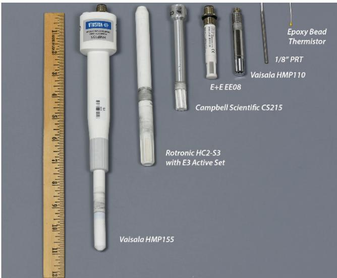
Fig. 8. Size comparison of some common temperature and relative humidity probes and two stand-alone temperature sensors (PRT and thermistor). Ruler scale is inches.
