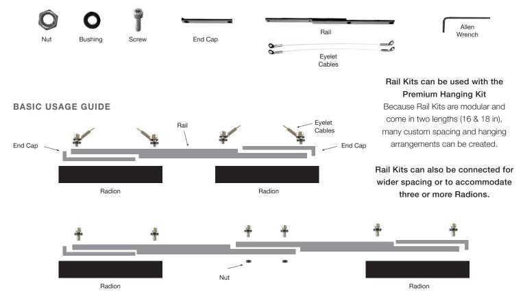
If you are using a Rail Kit in conjunction with the PREMIUM HANGING KIT, familiarize yourself with the hanging kit instructions before beginning. A minimum of ONE hanging kit per TWO Radions is recommended. Additionally, make sure that the hanging kit anchors are capable of supporting multiple Radion fixtures.
